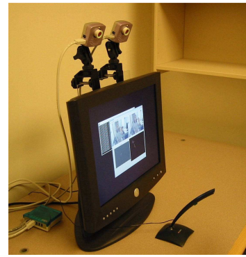
Fig. 4. Experimental Setup. Study participants were seated in front of a GWINDOWS-enabled display and an open microphone for speech recognition.
